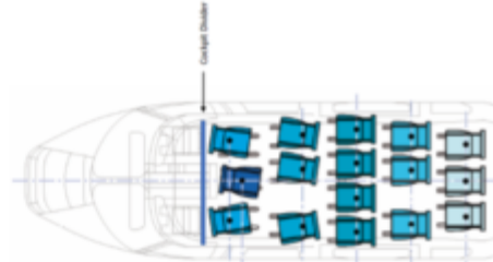
EC175 with cockpit-cabin divider:
